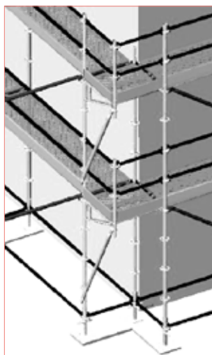
Fig. 2.13 – Corner made with three stands and a bracket
