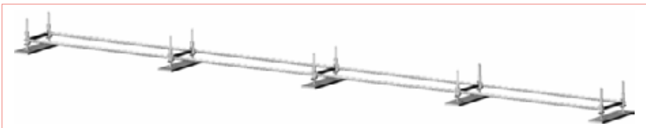
Fig. 2.32c – Stage 3 – Clamping of the primary elements
