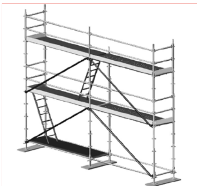
Fig. 2.11 – Example of scaffolding with side protection
