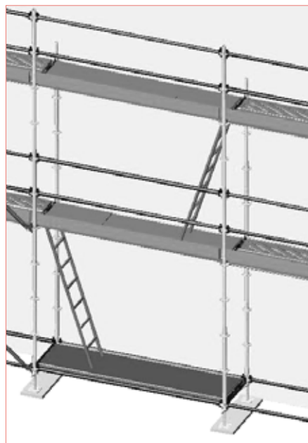
Fig. 2.23 – scaffolding entrance with the use of pass-by aluminium platforms equipped with aluminium ladders
