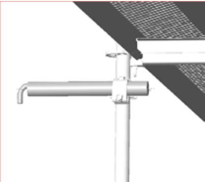
Fig. 2.18a – Anchoring of internal stands with single anchor
